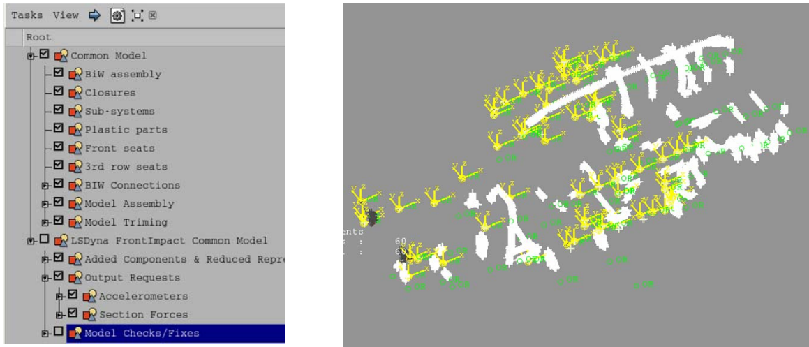
Fig.14. Accelerometers and sections created by Generic Entities
