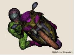
**Trends in CFD** Provide the right mesh for the right problem • Reduce the meshing bottleneck • Traditional Meshing Wrapperbased Time/ Meshing Manual Cartesian interaction Cut Cell **Design Process / Accuracy** Geometry "Quality" © 2006 ANSYS, Inc. All rights reserved. 28 ANSYS, Inc. Proprietary
