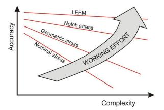
Figure 1 - Qualitative comparison of accuracy and effort for common fatigue assessment methods for welded structures (source: Marquis and Samuelsson [2, 3])
