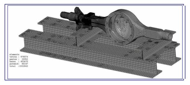
Figure 6 - Complete model - Test rig simulation
