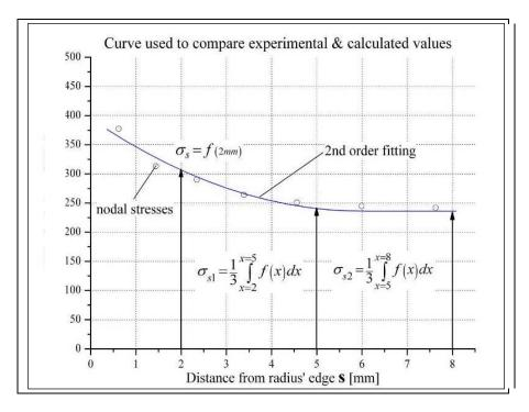
Figure 8 - Curve used to compare experimental and calculated values
