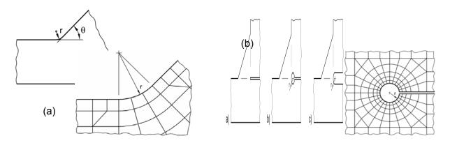
Figure 3 - Typical mesh for the notch stress analysis with elements having quadratic displacement function at the weld toe (a) and root (b) [5]
