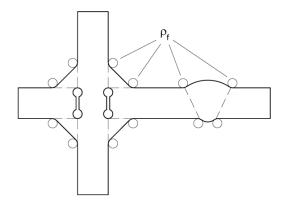
Figure 2 - Fictitious notch rounding (graph according to Hobbacher, 1996) [5]
