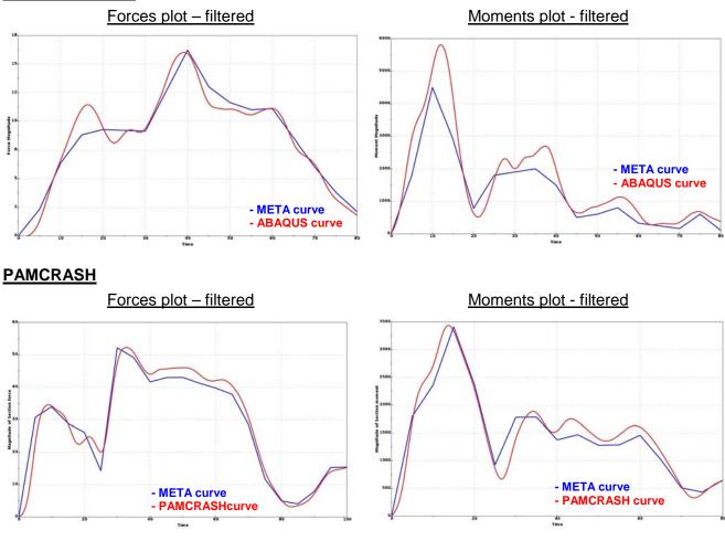
Having verified that the accuracy of the Forces and Moments calculated by META closely match those calculated by the solver, for existing sections, it is safe to conclude that this will be the case for Sections defined in META. This prevents the re-solving of crash models for sections not defined, making META a valuable Post-Solution calculator.
