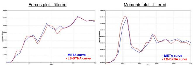
It is clear that the curves calculated by META closely follow those from the solver. Some peaks missed out are considered to be acceptable as the time interval for the calculation of the curve from META is much larger than that of the time history curve.
