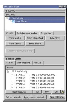
Sections can be created from *Visible* and *Identifed* elements, from *Groups* (including Node Sets defined in the input deck), from existing *Planes* (including Sections defined in the input deck) and by specifying filtering criteria in the *Advanced Filter* tool of META.
