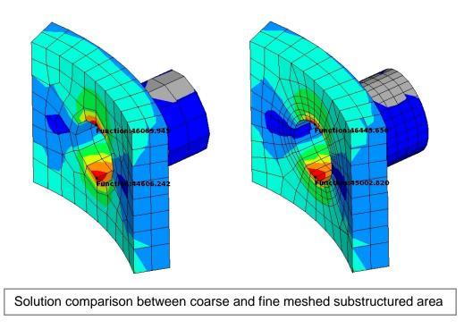
It is clear how the fine mesh gives a more accurate insight of the behaviour of the model compared to the coarse mesh model.
