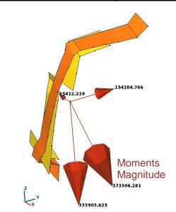
The vectors originate from the geometrical centre of the nodes assigned to the section. Subsequently, the Force and Moment results calculated by META are plotted against those of the LS-Dyna time history:
