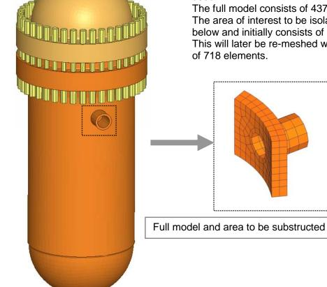
Through the Sections tool of META, it is possible to calculate, from the full model's solution, the Freebody Loads on the external nodes of the isolated area of interest:
