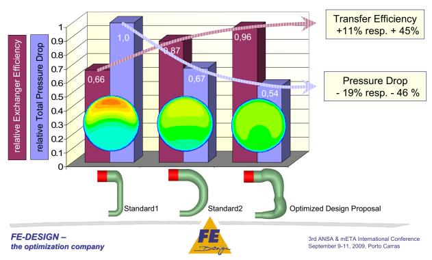
• Cross sectional velocity uniformity and heat exchanger efficiency
