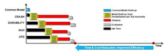
Figure 11 – Profile of an improved CAE workflow
