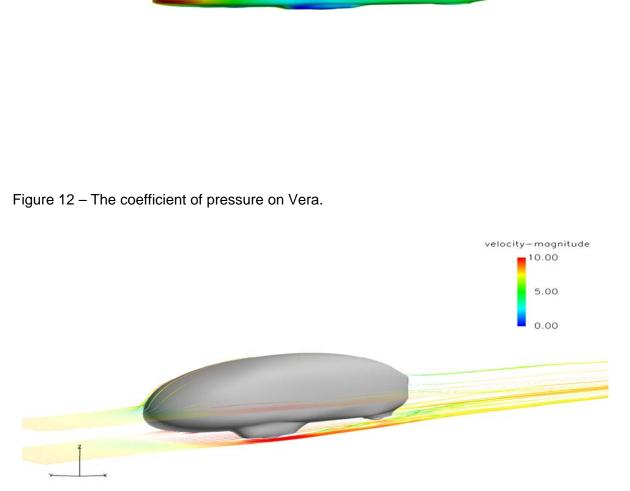
Figure 13 – Streamlines visualizing the flow field around Vera.
