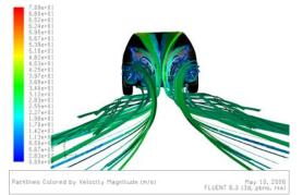
Figure 4 – Streamlines in the wake of the VRAK model.
