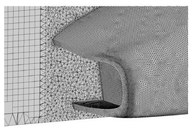
Figure 7 – The mesh at the front section of the car.
