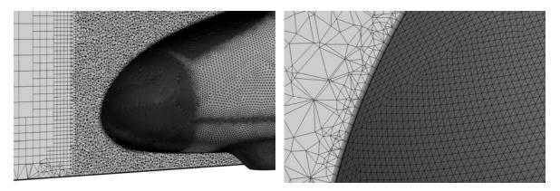
Figure 11 - A cut-out of the mesh. On the right a zoom-in image displays the 10 layers of prism cells.
