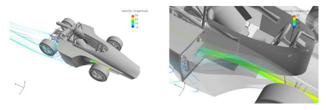
Figure 9 – Streamlines illustrating the improved cooling flow.
