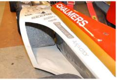
Figure 6 – The 2997 Chalmers formula student car and on the right a close-up on the right sidepod where the radiator is located.
