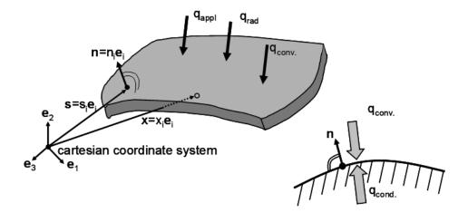
Fig.2 Solid structure with boundary conditions
