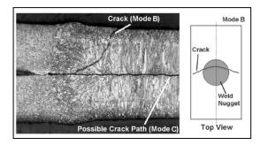
Figure 4 – nugget failure (Yi Gao[3])
