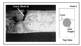
Figure 3 **(**sheet failure (Yi Gao[3])
