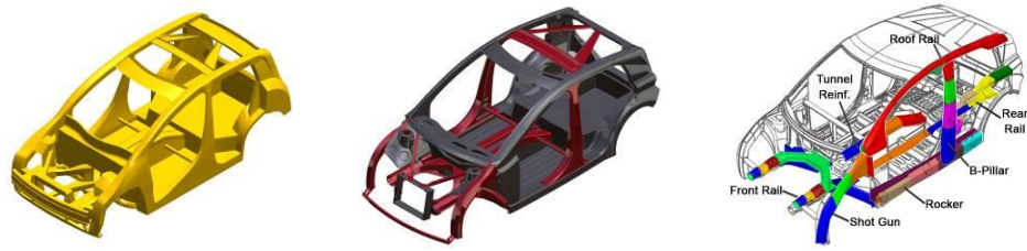
Figure 6: a-LF3G optimization, b-reference body structure and c-structural sub-systems
