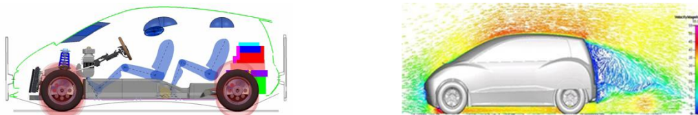
Figure 3: BEV packaging theme and aerodynamic study
