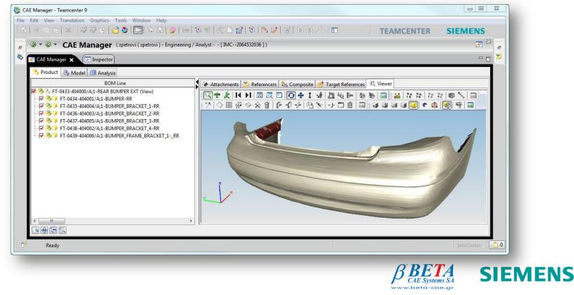
This use case consists to open directly a Product Structure into ANSA without making use of a CAE Structure. The steps to send the data to ANSA is identical as in the first use case.
