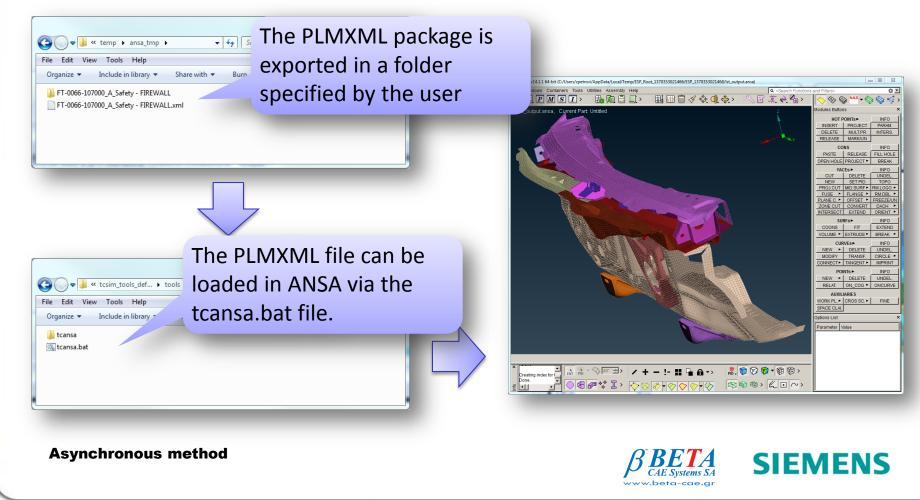
• The data can be sent to ANSA synchronously or asynchronously
