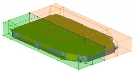
Figure 2 – Basic Box Morphing Conceptual Parameterisation of a Battery Pack
