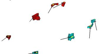
Figure 5: Study to evaluate relationship between load cases and design variables. One iteration of forces acting on battery pack fixing points
