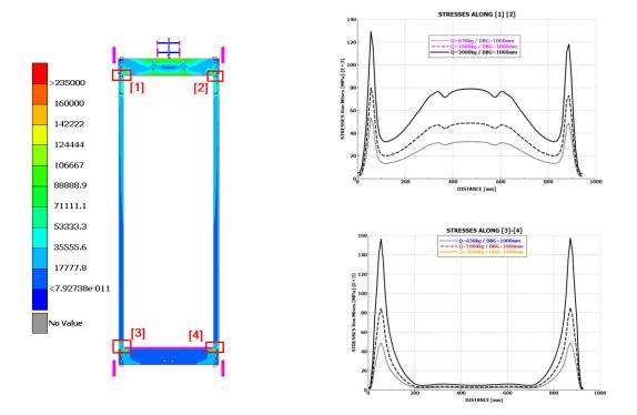
Figure 7 – Stress field diagram of the complete counter weight frame of a traction elevator (left) and the changes of stresses along DBG as a function of passenger cabin rated load (right)
