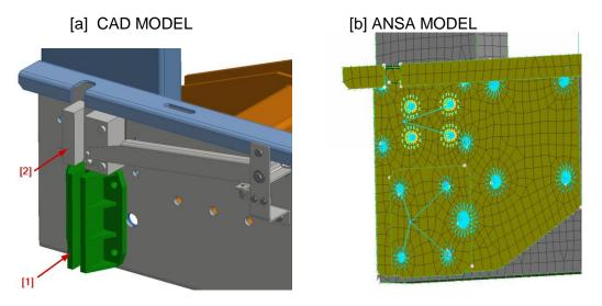
Figure 4 – Example of FEA models developed to simulate [1] guidance shoe and [2] safety gear. Left their 3D CAD geometries, right the equivalent automated created RBE2 models in ANSA.
