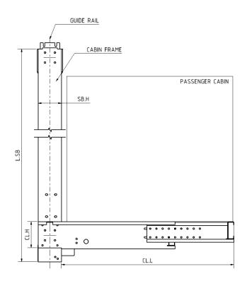
Figure 2 – Simplified assembly of car frame and a passenger cabin. The free length of the cantilever CL.L is the main design parameter used to asses the mechanical behaviour of a car frame.
