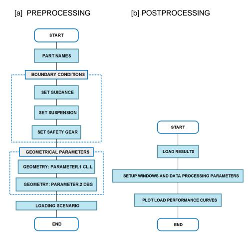
Figure 3 – Workflow chart for both preprocessing [a] and postprocessing [b]
