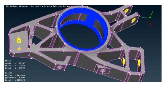
Figure 2 - Forces (yellow) applied on the surface of the holes – constraints applied on the bearings surface (blue)
