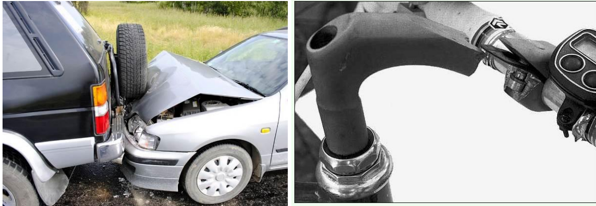
Figure 1 – Left image: in a crash or overload situation, the relation between the loading and the resulting deformation is often obvious to the everyday customer. Right image: fatigue failure often comes unexpectedly to a customer, without any obvious coupling to the current loading. (Failure of a bicycle handlebar stem).
