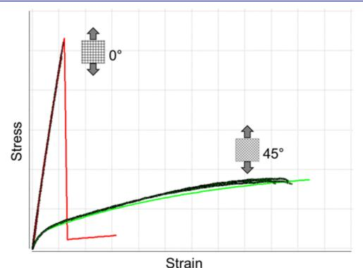
Figure 1 – Effect of woven laminate fiber orientation on stress-strain curve. (5)
