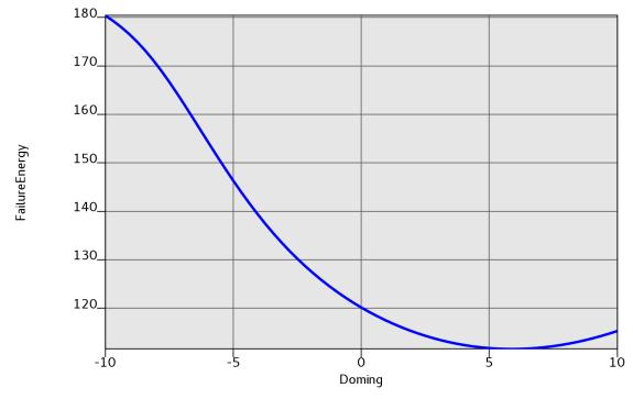
Figure 8 – Effect of Doming on Energy to Failure
