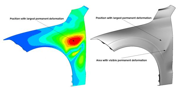
Figure 7 – Left: Current evaluation using contour plot. Right: Evaluation using Meta render view mode.
