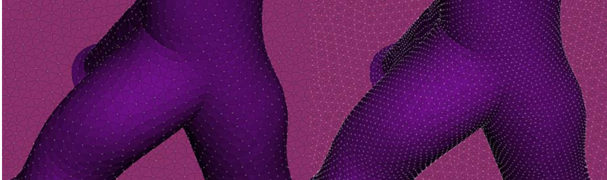
Figure 3 – Surface mesh before (left) and after (right) add a point in the middle of the edges.
