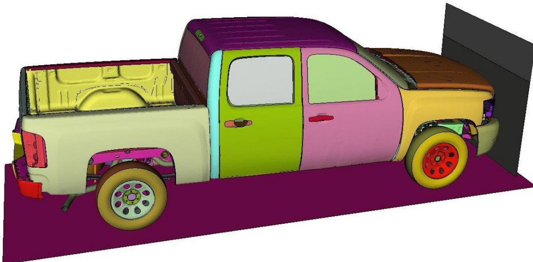
Fig.1: Snapshot of a simulation run of the Chevrolet Silverado before the crash.
