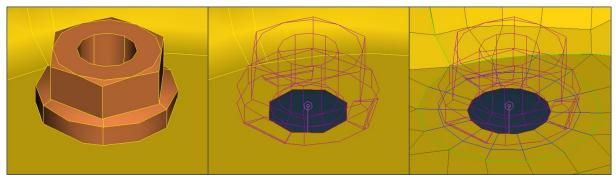
Figure 2 - Example on automated model preparation from CAD to FE-representation
