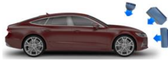
Figure 3 – Pedestrian protection tests scheme.
