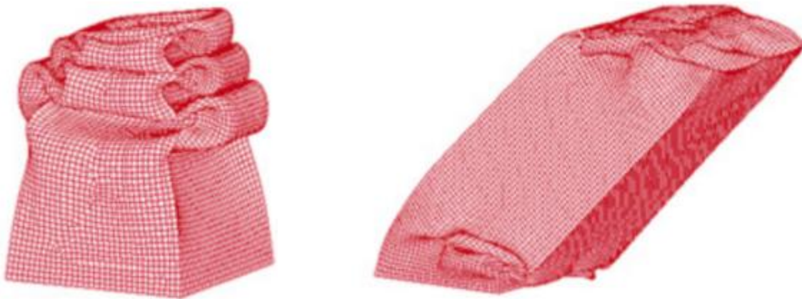
Figure 13 – Examples of crashbox deformation, crushing (left side) and lateral bending (right side).
