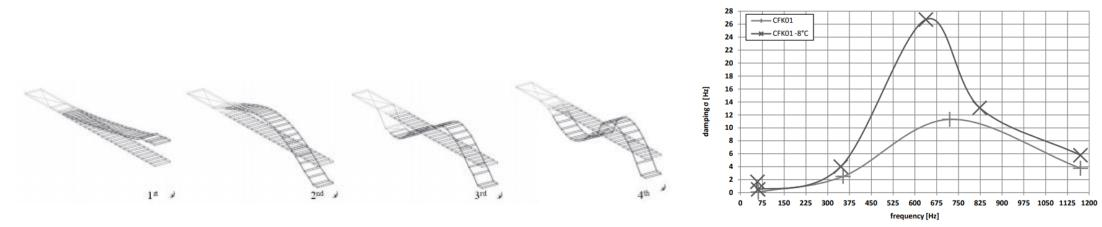
Mode Shapes of CFRP Leaf Spring
