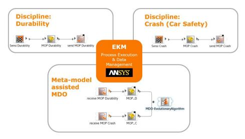
Figure 2 – Conceptual view on the exchange of meta-models via EKM (Simulation Data and Process Management) solution between individual disciplines and the meta-model assisted MDO process.
