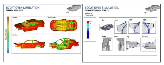
Figure 2 – Exemplary presentation of thermal and thermomechanical simulation results.
