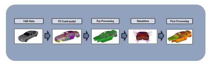
Figure 1 – Steps taken in the simulation process with respect to the paint shop.
