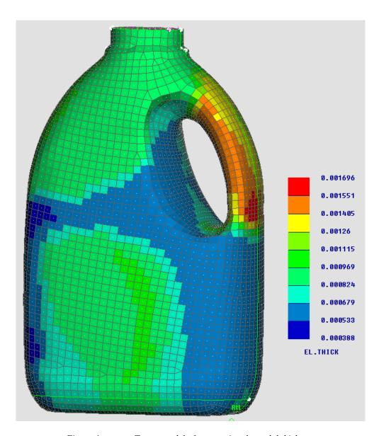
Figure 4: Target model after mapping the nodal thickness
