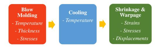
Figure 2: Blow Forming Simulation
