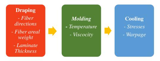
Figure 5: Typical Resin Transfer Molding (RTM) simulation
