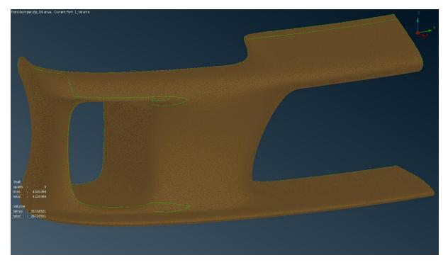
Figure 3: Meshed bumper CAD model (front view)
