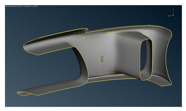
Figure 2: Bumper CAD model (rear view) with patch antenna placed behind it
