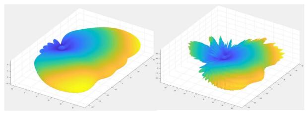
Figure 4: 3D radiation pattern of the antenna in free space (left) and behind the bumper (right)
