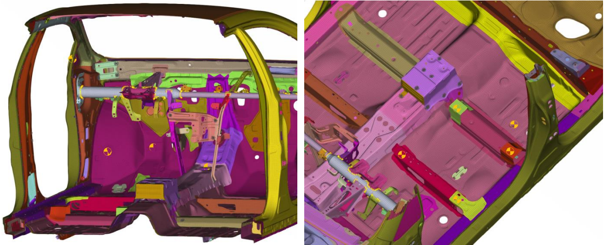
Figure 7: Intrusion measurement (left), Acceleration measurement (right)
