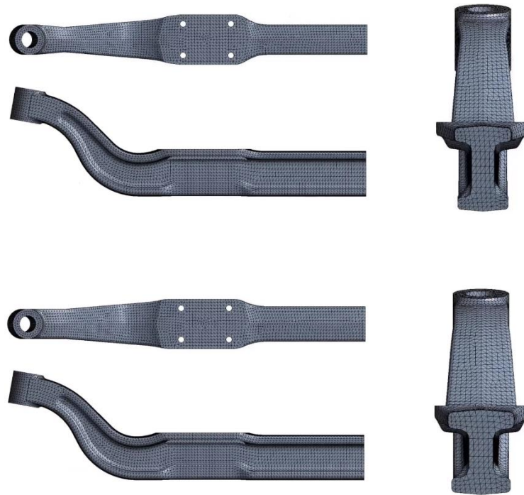
Figure 10: Optimal (upper) vs. initial geometry (bottom)
