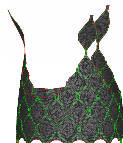
SKIRT 32,883 TRIANGULAR MEMBRANE ELEMENTS
