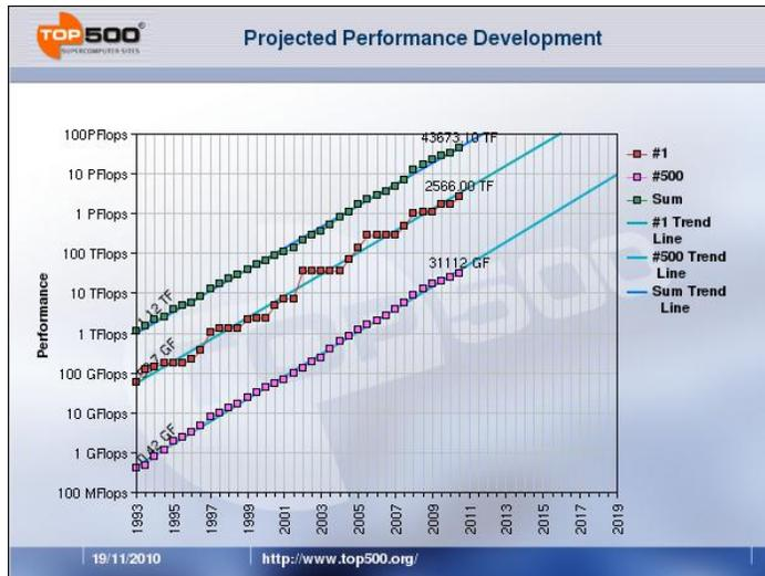
Figure 2 - Computing capacity growth at Top 500 sites worldwide
