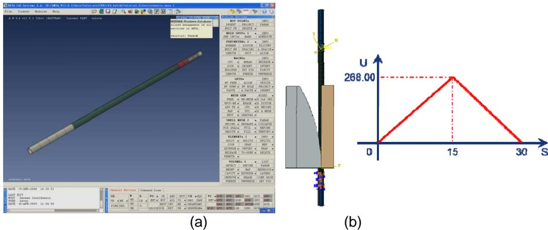
Fig. 2 The mesh of coiled tube (a) and boundary conditions (b)
