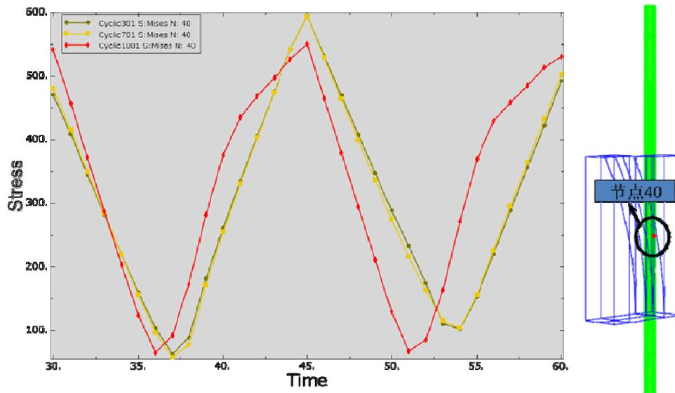
Fig. 6 The stress value change with time after the different cyclic loadings
