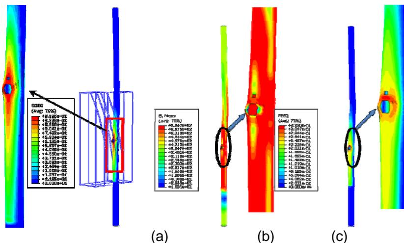
Fig. 7 The SDEG contours of model with inner pressure after the 260 cyclic loadings (a); The stress contours (b) and PEEQ contours (c)
