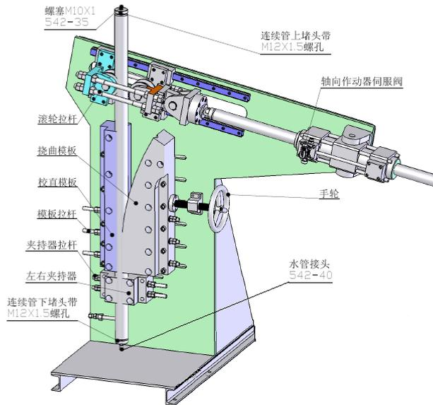
Fig. 1 The experimental facility of testing the fatigue life of coiled tube
