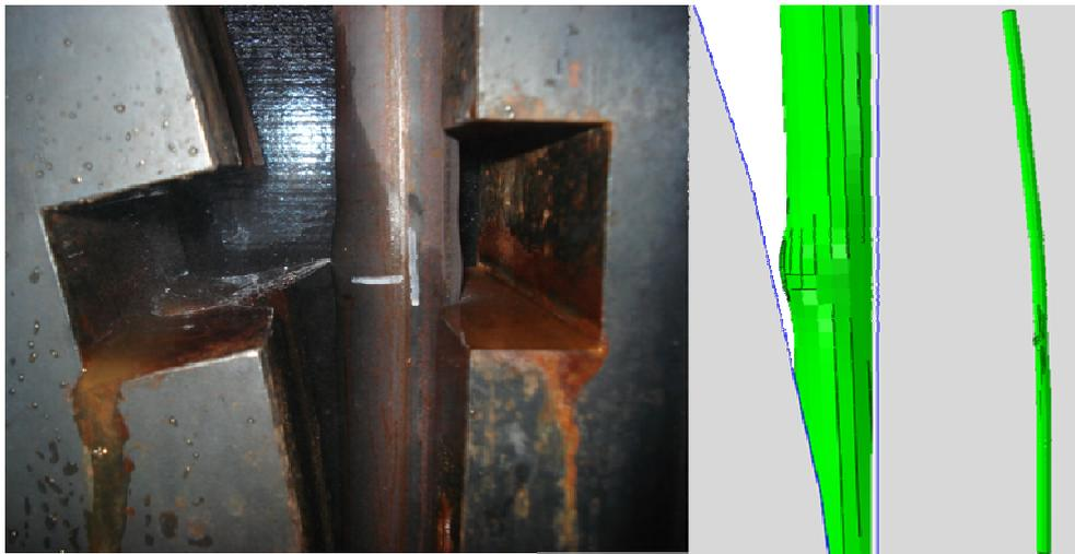
Fig. 8 Comparison of the experimental results and the simulation
