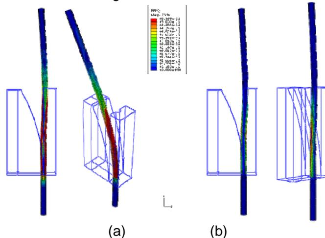
Fig. 4 The Mises contours (a) and the equivalent plastic strain (b) under one cycle movement
