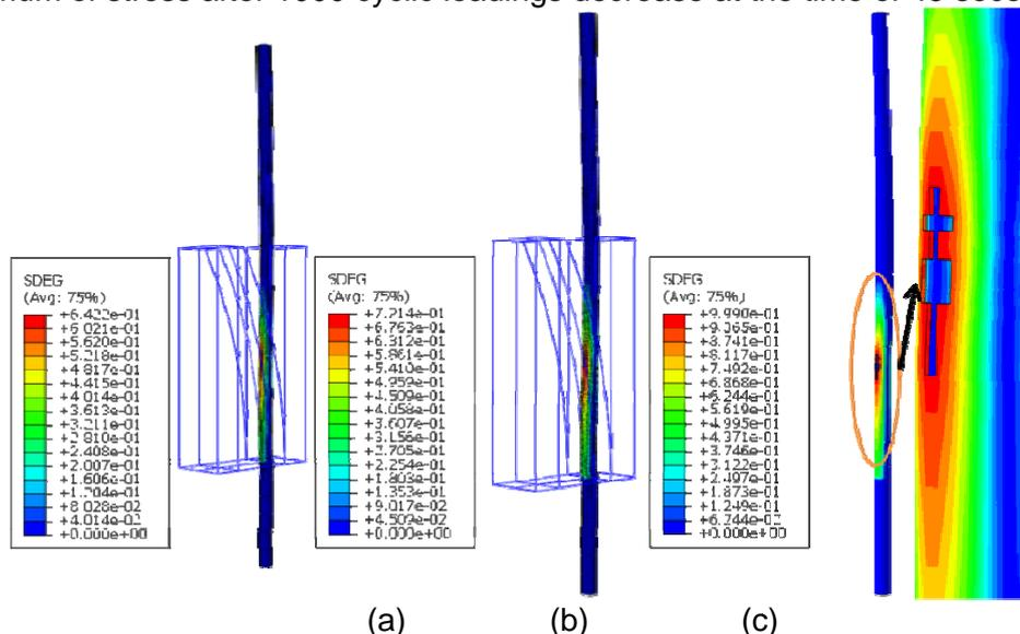
Fig. 5 The SDEG contours after the 300 (a), 700 (b) and 1000(c) cyclic loadings
