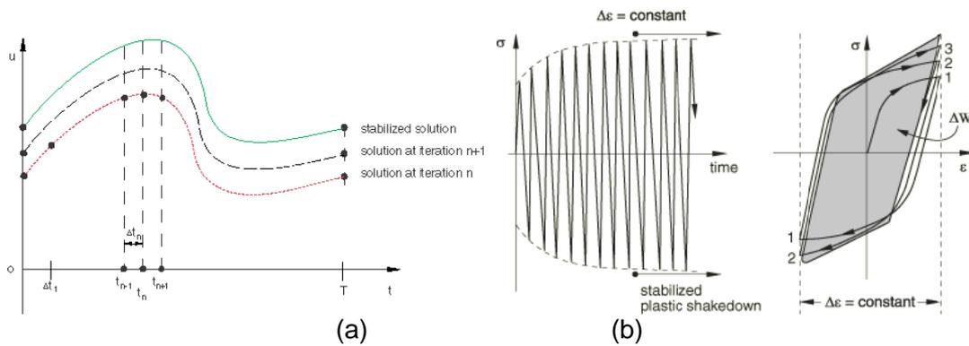
Fig. 3 A displacement function at all times  $t$  during a load cycle with period  $T$  at different iterations (a) and Plastic shakedown in a direct cyclic analysis (b)
