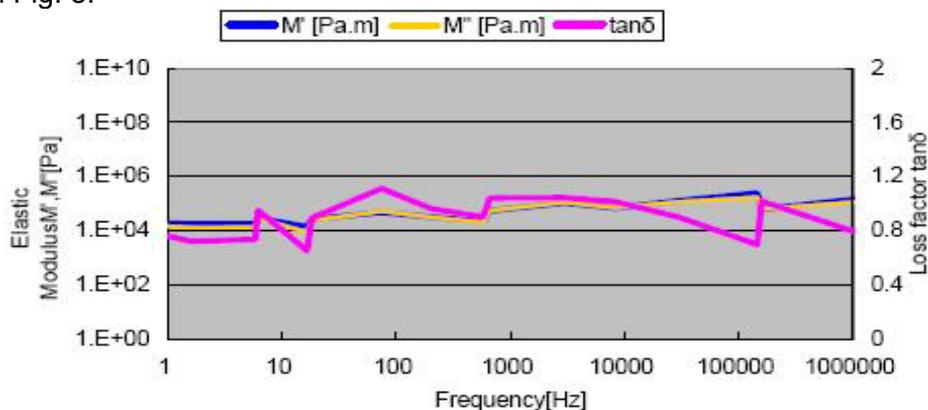
Fig. 8 Tested storage modulus and loss modulus for the material.
