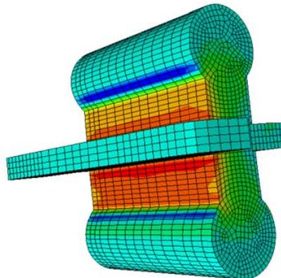
Fig. 5 Stress contour for a plastic insert during back face drop.
