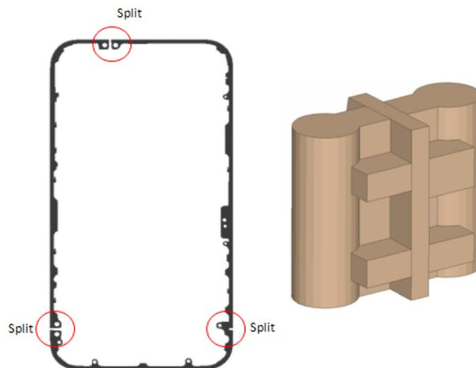
Fig. 1 The split band and plastic insert.
