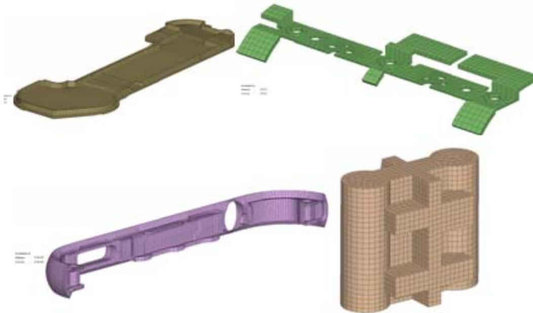
Fig. 3 Hex mesh for some components.
