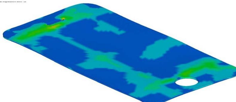
Fig. 6 Stress contour for the cover glass during back face drop.
