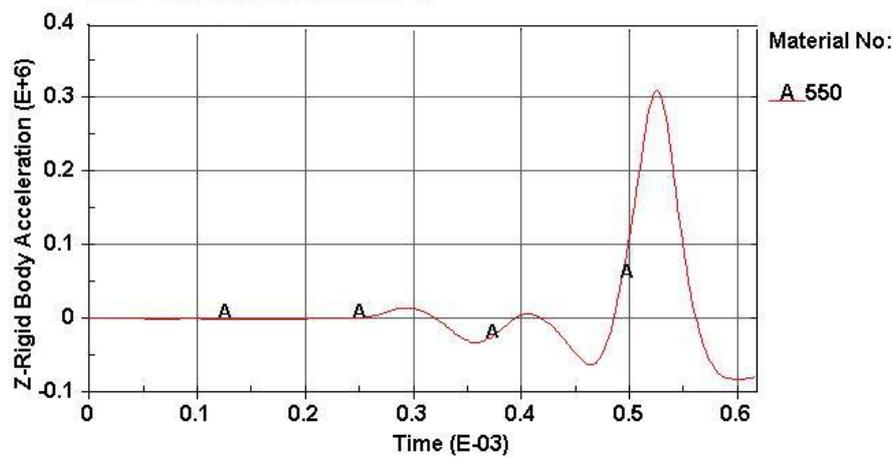
Fig. 9 Acceleration history of the camera lens during face tilt drop.
