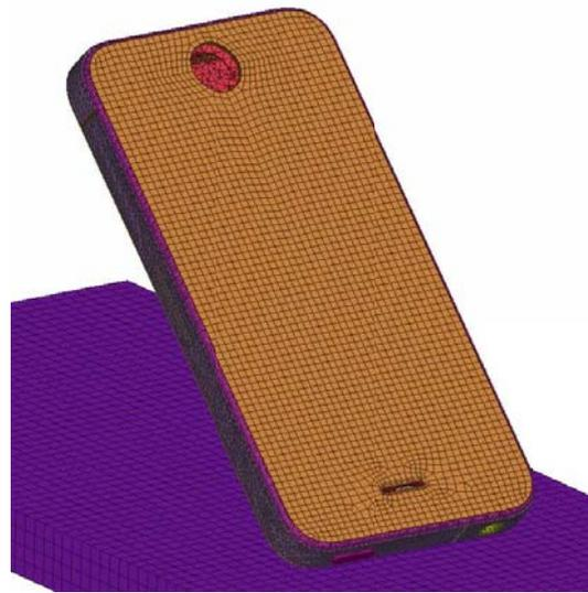
Fig. 4 FE model of the assembly.
