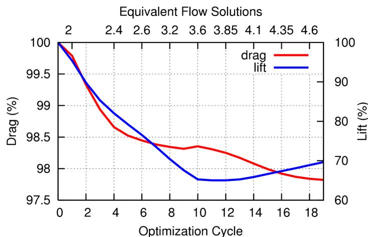
**Fig. 5:** Drag and lift evolution during the one-shot optimization. After 10 cycles, the step size was reduced by one half. Note that the whole optimization required a computational effort of less than 5 equivalent flow solutions (see upper x-axis).
