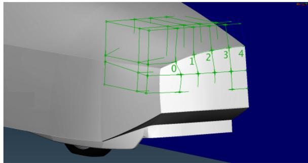
**Fig. 4:** Morphing boxes and control points for the rear spoiler area.
