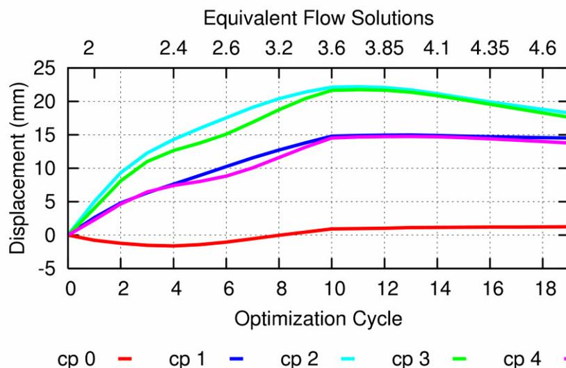
**Fig. 7:** The evolution of the control point coordinates during the one-shot optimization (cf. Fig. 4 for the respective position of the control points cp0 to cp4).
