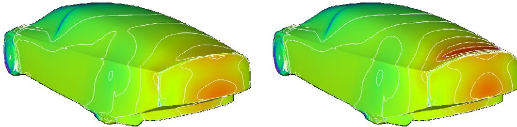
**Fig. 6:** Pressure contours on the car surface before (left) and after the optimization (right). Note the large footprint of the rear spoiler on the right picture.
