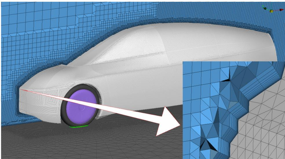
**Fig. 2:** The computational mesh generated by ANSA.
