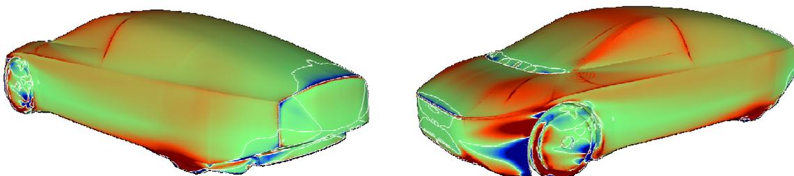
**Fig. 3:** Drag sensitivity maps for the L1. Strong red and blue areas pinpoint those regions on the car surface, where shape changes have a significant impact on the aerodynamic drag, whereas greenish areas are rather insensitive. The sensitivity map also provides information on the direction of the favourable shape change: red areas have to be moved inwards and blue areas outwards in order to reduce drag.
