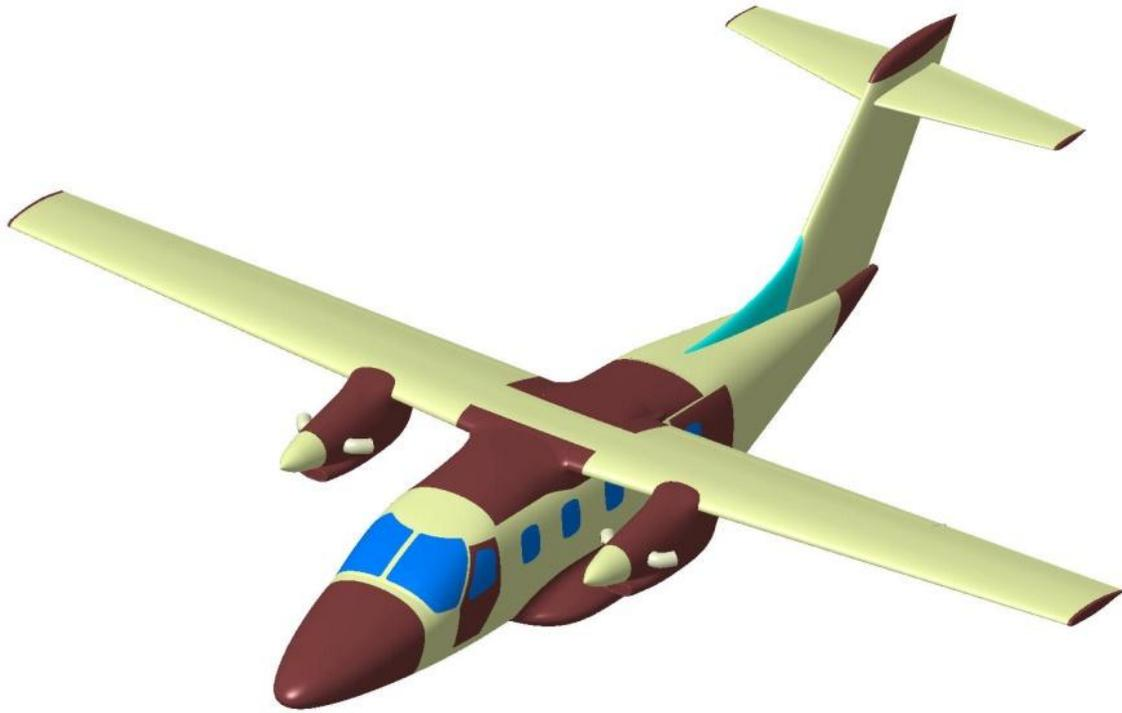
Figure 2 – Material diversity of EV55 airframe skin: basic metallic structure is yellow, CFC parts are brown, plexiglass windows' filling is blue and glass fibre composite (GFC) is green.
