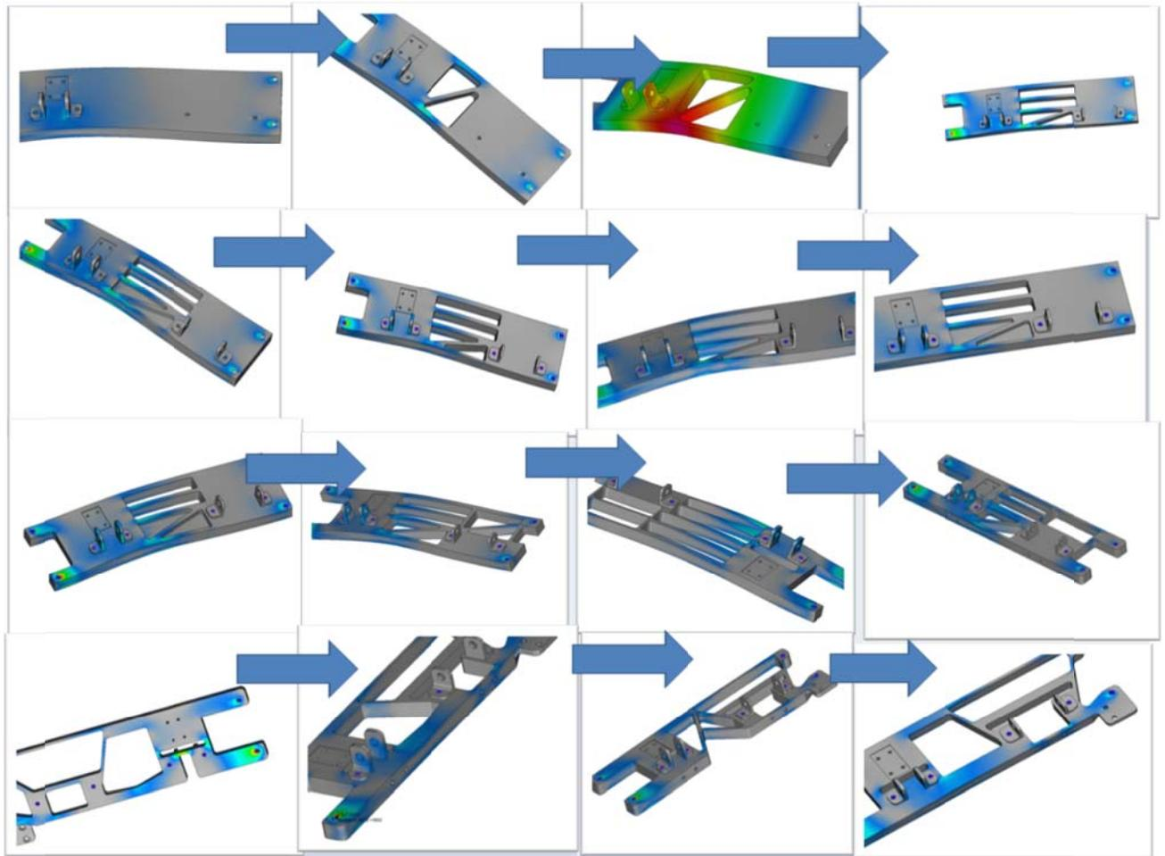
Figure 4 – Design optimization of the pedal box, manually and software assisted (bottom right).
