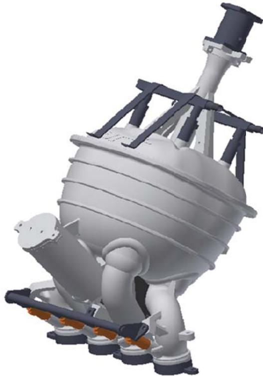
Figure 6 - 3D view of the new intake manifold.
