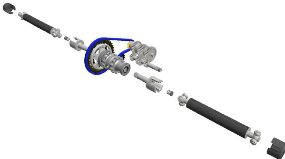
Figure 2 - 3D view of drive-train system
