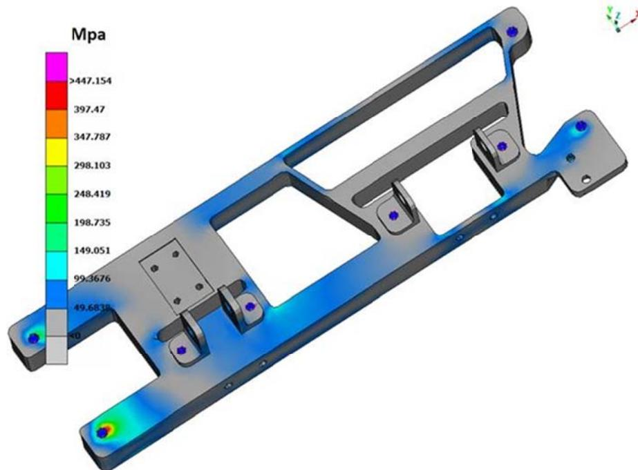
Figure 5 - von Mises stress distribution in the adjustable pedal box, as defined for the optimum pedal box design.
