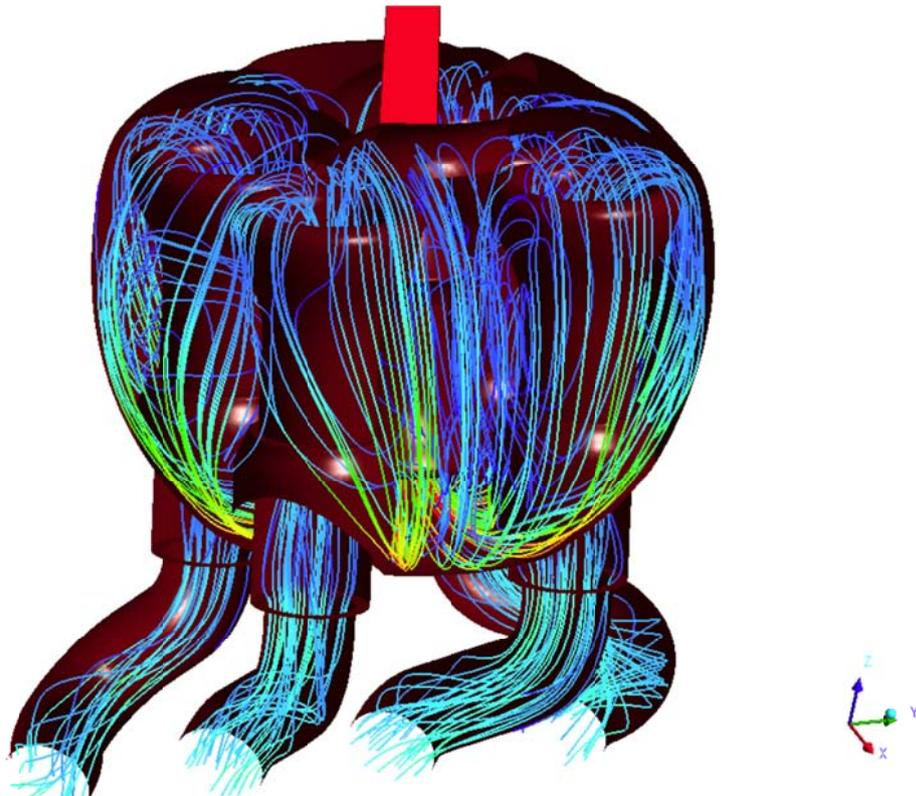
Figure 8 – Visualised result of CFD analysis of the intake plenum.
