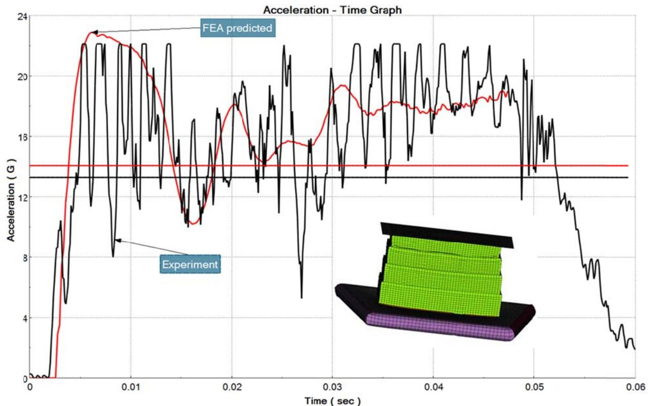
Figure 9 – Impact attenuator dynamic simulation model and acceleration graph – comparison with the tested acceleration.
