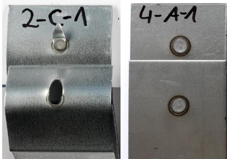
Figure 7 – Nugget pullout and interfacial fracture mode
