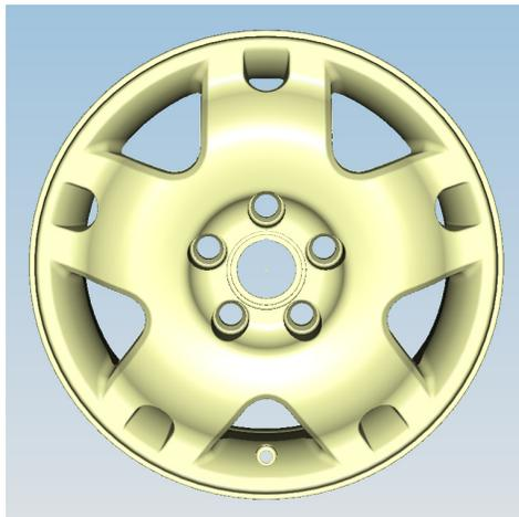
Figure 2 - CAD model of aluminium alloy wheel.
