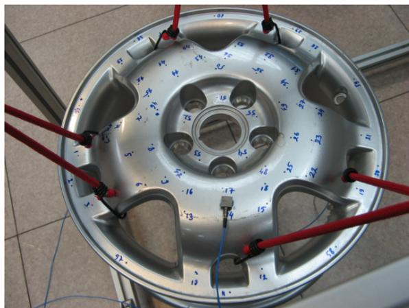
Figure 10 - Accelerometer position.
