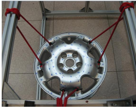
Figure 5 - Determined 100 points on free-free boundary condition simulated structure.
