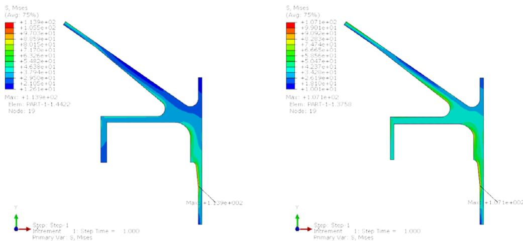
Figure 4 –section before and after optimization
