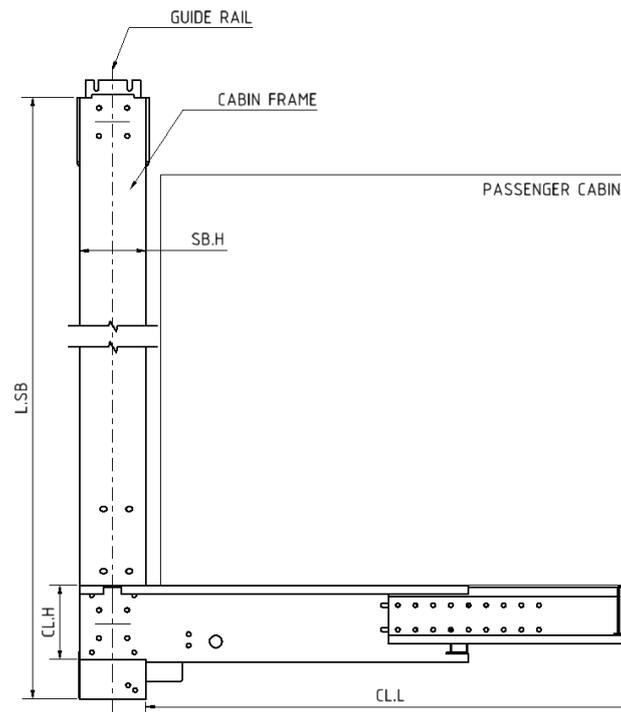
Figure 2 – Simplified assembly of car frame and a passenger cabin. The free length of the cantilever CL.L is the main design parameter used to assess the mechanical behaviour of a car frame.
