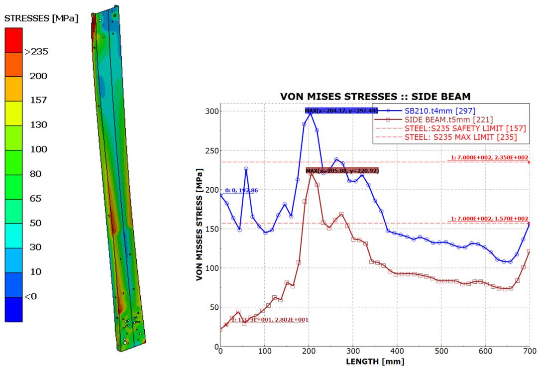
Figure 6 – Stress field diagram of the side beam (left) and changes of Von Mises stresses as a function of side beam length, using the beam thickness as a parameter.
