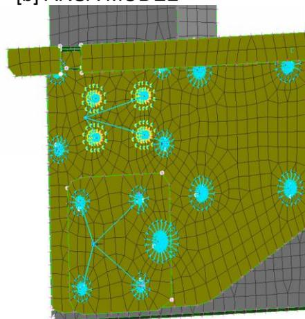
Figure 4 – Example of FEA models developed to simulate [1] guidance shoe and [2] safety gear. Left their 3D CAD geometries, right the equivalent automated created RBE2 models in ANSA.
