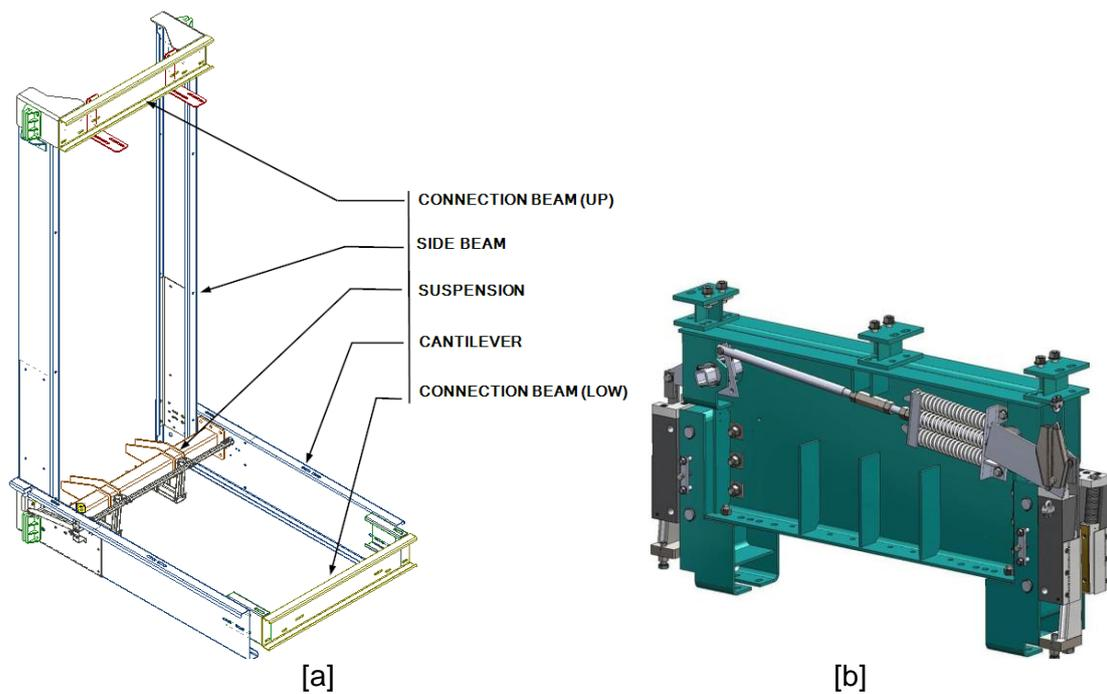
Figure 1 – [a] Elevator cabin frame and its main parts (courtesy of TELCO, complete elevators) [b] One direction safety gear mechanism (courtesy of Wittur, complete elevators and elevator parts)
