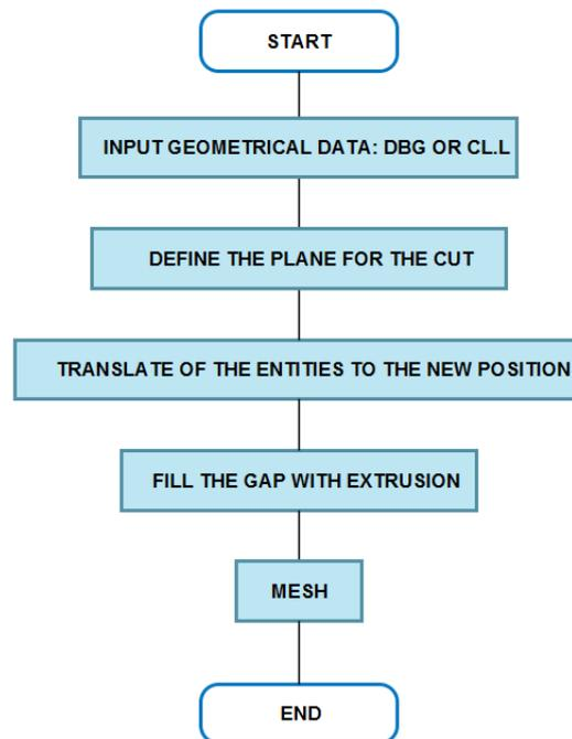
Figure 5 – Workflow chart for parametrization of the geometry.
