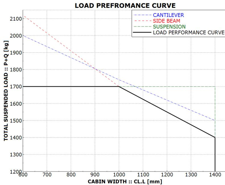
Figure 8 – Load performance of each component of the elevator
