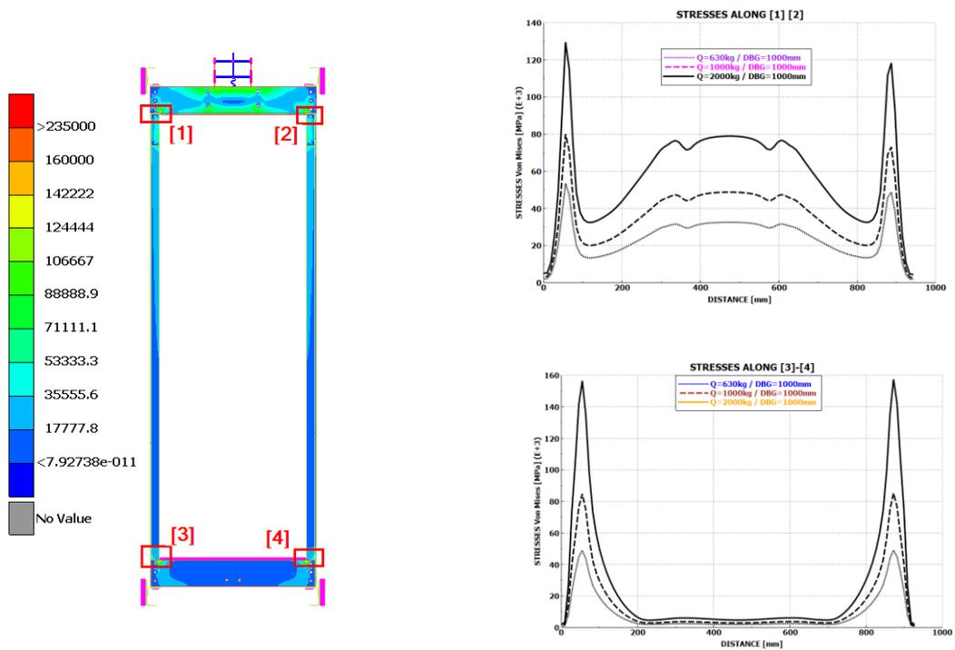
Figure 7 – Stress field diagram of the complete counter weight frame of a traction elevator (left) and the changes of stresses along DBG as a function of passenger cabin rated load (right)
