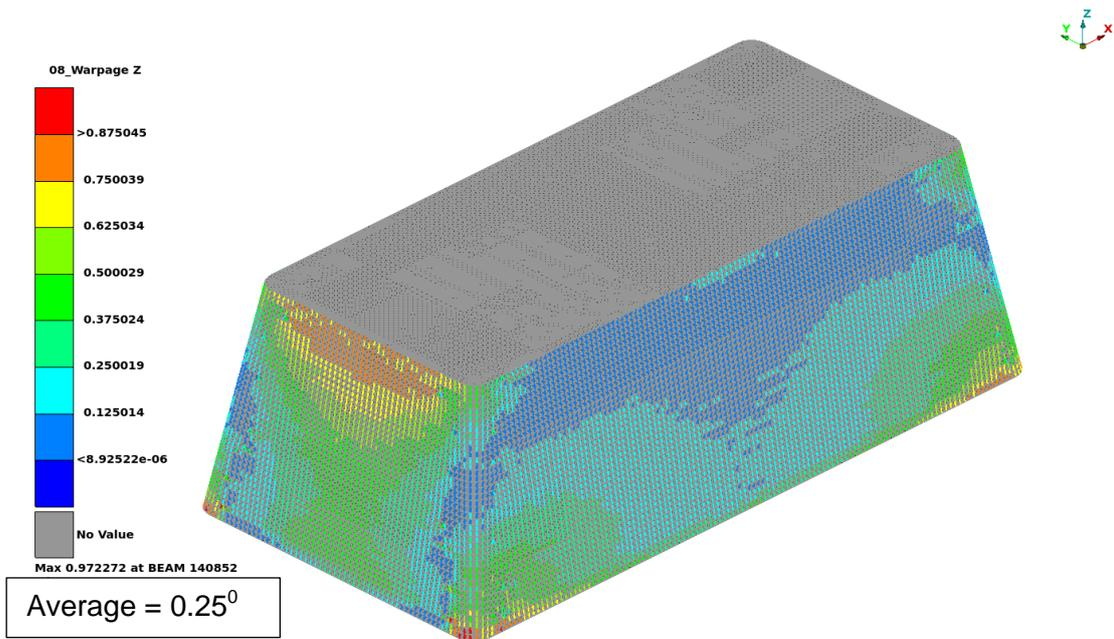
Figure 11. Contour of rotation (warpage) with respect to Z axis for beams in Z direction
