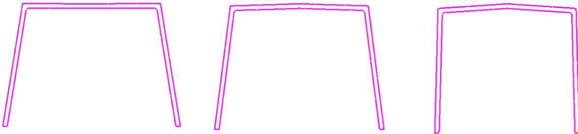
Figure 2. Example of warpage of a 2-D section due to distortion
