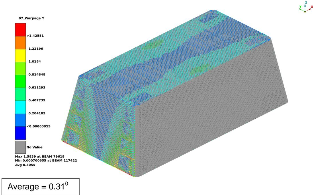
Figure 10. Contour of rotation (warpage) with respect to Y axis for beams in Y direction
