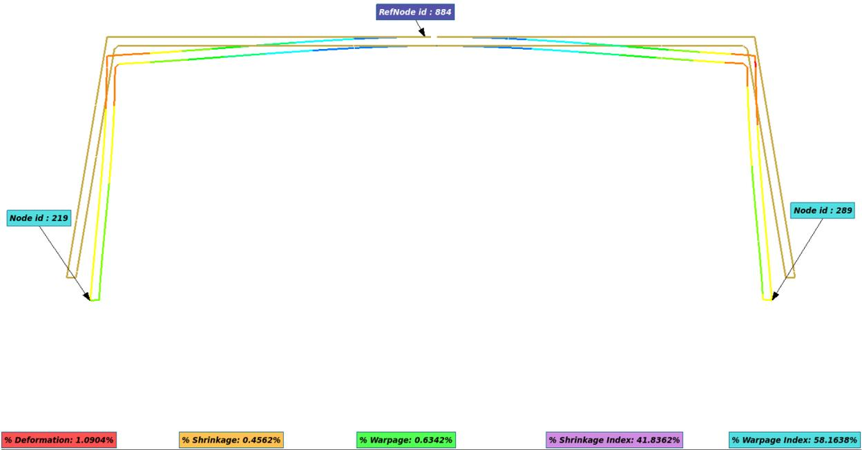
Figure 15. Warpage of a section across length of the mouse coffin
