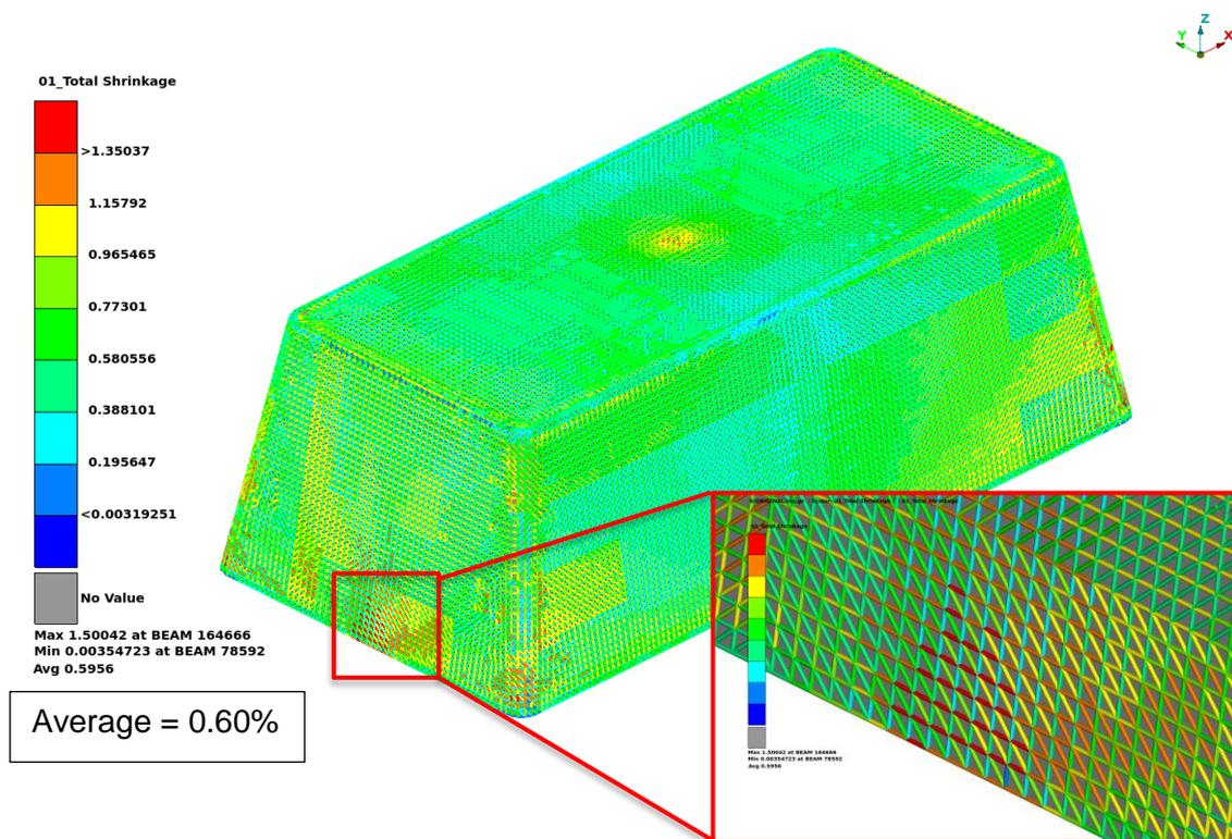
Figure 4. Shrinkage contour plot on mouse coffin
