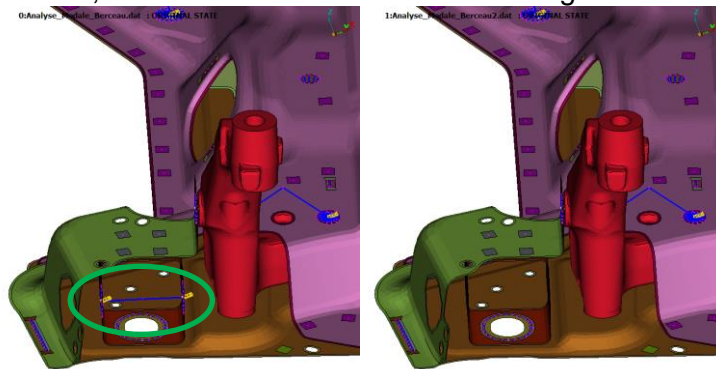
Figure 13 – Reference model (left) and modified model (right). A connexion is missing in the modified model.
