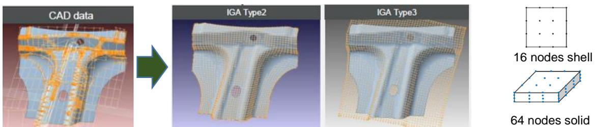
Figure 1 – Isogeometric models made by NURBS generator tool and generated elements with high order shape function
