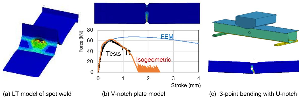
Figure 3 – Fracture and crack propagation of Isogeometric models
