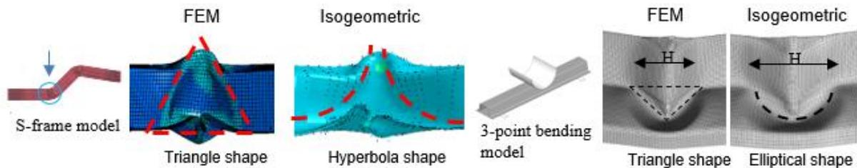
Figure 2 – Local deformation of S-frame and 3-point bending model
