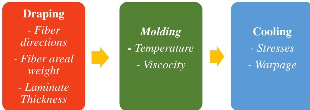
Figure 5: Typical Resin Transfer Molding (RTM) simulation
