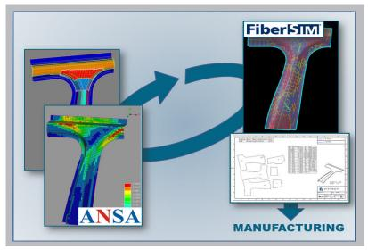
The FiberSIM® Analysis Interface™ drives analysis from the same single CAD master model that is used for design and manufacturing. This permits engineers to analyze a part in its to-be-manufactured state.
