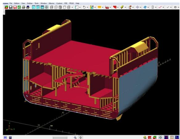
Some geometry clean-up and idealizations are applied in FORAN to facilitate the meshing process. The STEP file, then, is imported to ANSA. A special ANSA script parses the xml file and applies the necessary information to the model. The plate parts of the FORAN file are
