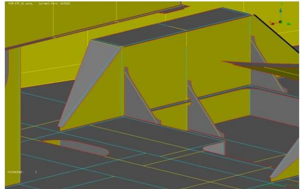
Among the additional numerous capabilities in handling geometrical features, holes and welding cuts can be automatically filled and cracks can be closed.
