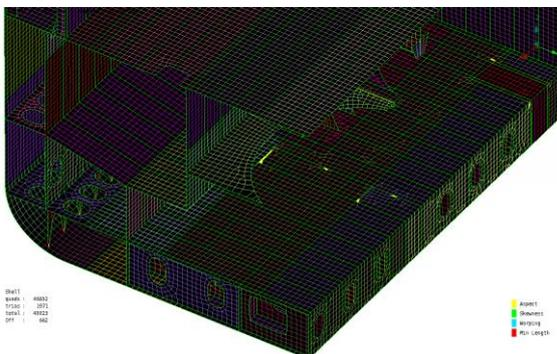
The profile parts can be exported by FORAN as beams or surfaces. In this case,
