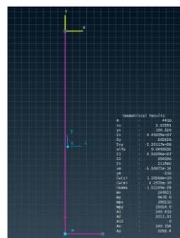
When the user wants to create a stiffener of a specific cross section, he can select this cross section from the database. Then, the edge of the model
