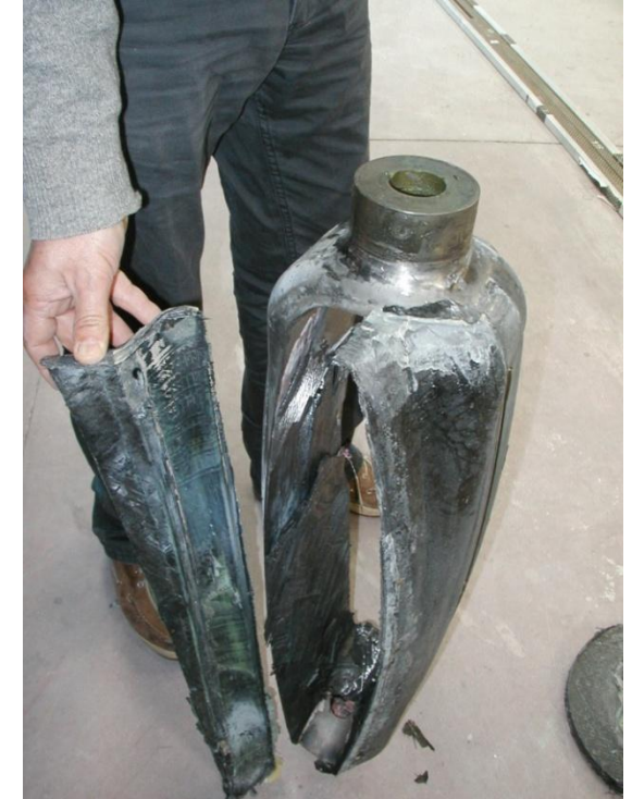
Keel remaining parts after failure (titanium belt)
