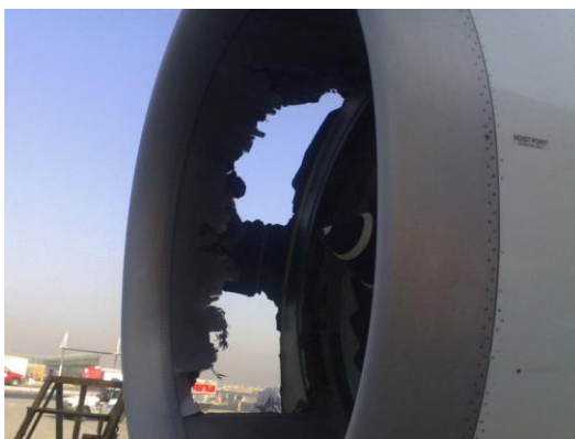
Figure 1 – After the Bird hit first on the Engine and 2 nd hit on Engine Casing [4]
