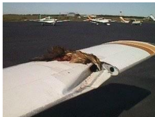
Figure 2 – After the Birdstrike on Aircraft wing [4]
