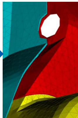
Final watertight mesh with all necessary details
