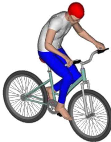
Figure 9: Positioning of THUMS on configurations via combining HBM Articulation tool and Bike Configurator Tool
