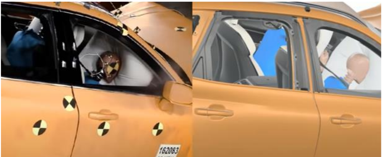
Figure 2: Simulation vs Test video. (Courtesy of VOLVO Safety Cente)
