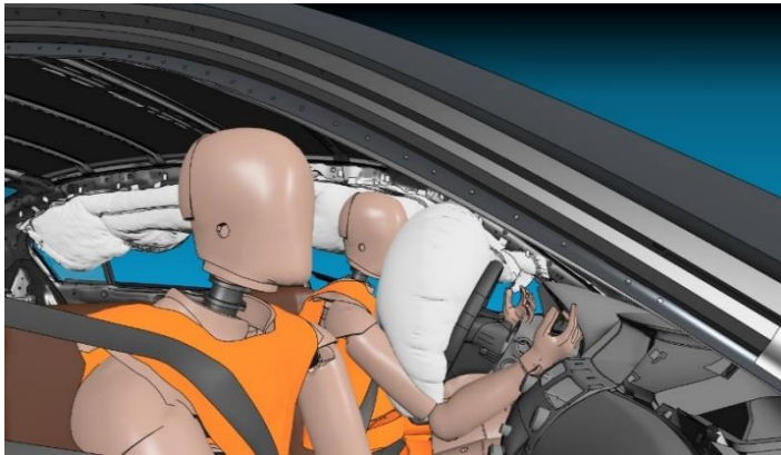
Figure 1: Front Impact simulation
